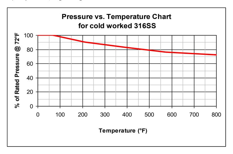
**Note:** The above pressure temperature chart is for 316 cold worked materials, this chart does not account for the temperature rating of packing or o-ring material which could be the limiting factor. Contact factory for other material limitations.
