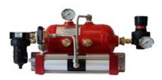
This MAXPRO air driven air amplifier system was designed for smaller point-of-use shop air applications that require higher air pressure for successful operation. This approach allows air compressors that serve an entire shop to run at a lower, more efficient pressure level while the air amplifier provides the higher pressure needed to run specific equipment.
