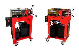
Model #MTCAT – Quickly cones and threads 1/4", 3/8", 9/16", 3/4" and 1" Medium Pressure and 1/4", 3/8", and 9/16" High Pressure Tubing. US Patent #9,015,915, CE Mark
